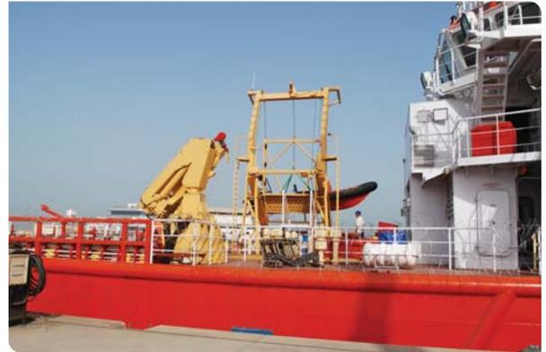
Davit and crane installed on top of new module deck
